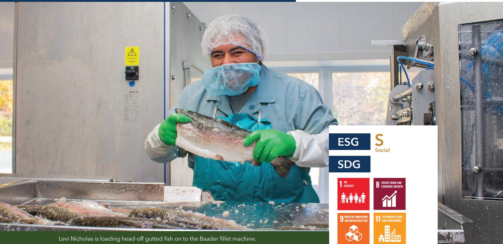
Levi Nicholas is loading head-off gutted fish on to the Baader fillet machine.
